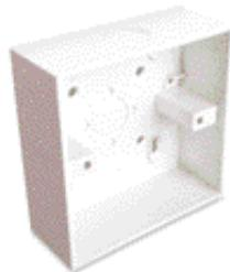
**SHB 1**, distribution and outlet box, surface type, single gang, according to British Standard BS 4662; white (RAL 9010), mounting screw spacing 60mm, lugs with brass inserts, knock-outs for 1 conduit and 1 trunking
