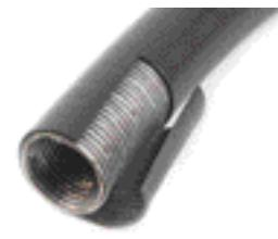
**KFR**, pliable steel conduit, heavy gauge; with insulating intermediate layer and plastic coating, in coils of 25m
