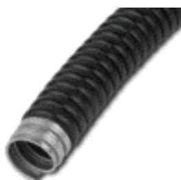
**MVK**, flexible metal conduit, medium gauge; zinc plated sheet steel, helically wound, with plastic coating from PVC-P, black (RAL 9005) in coils of 100m, 50m resp. 25m
