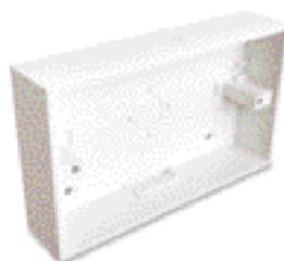
**SHB 2**, distribution and outlet box, surface type, twin gang, according to British Standard BS 4662; white (RAL 9010), mounting screw spacing 60mm, lugs with brass inserts, knock-outs for 1 conduit and 1 trunking
