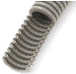
**FXP-Turbo®**, pliable conduit medium gauge, corrugated, with sectional corrugation; grey (RAL 7037), in coils of 50m resp. 25m
